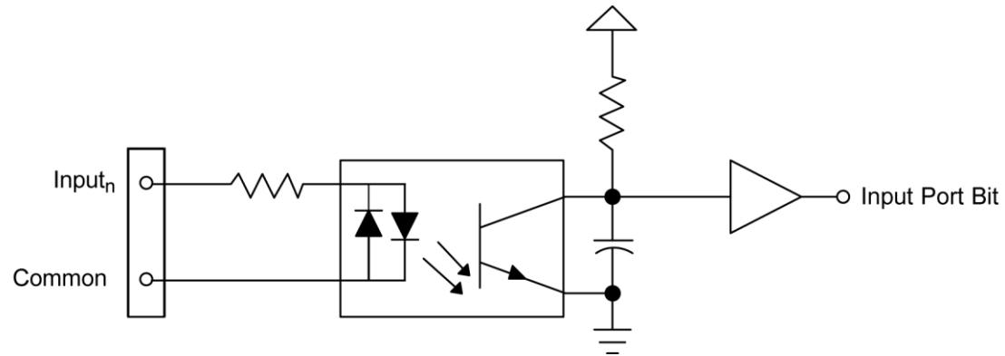
In the above circuit diagram, Input<sub>n</sub> is one of the two Input Pair Pins from the table labeled Input Ports Pin Assignments. Common is the other pin listed in the Input Pair Pins entry. The polarity of the pair does not matter.
