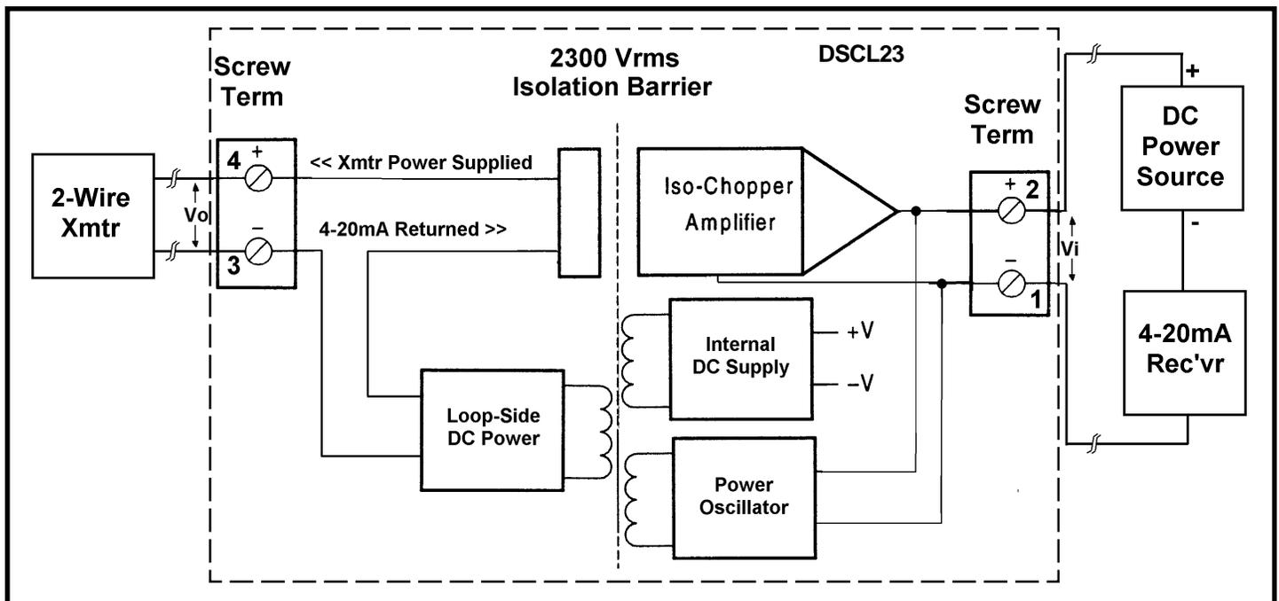
Figure 1: DSCL23-01 Block Diagram, Single Channel Model
