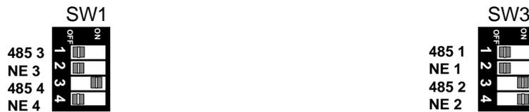
Figure 2: RS422/485 Interface Configuration
